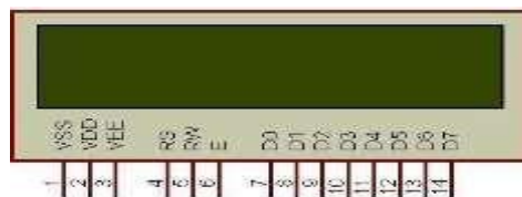
Fig 8 Character LCD type HD44780 Pin diagram
