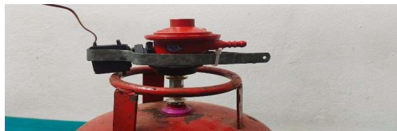
Fig.5: Servo Motor Integration to the LPG gas Cylinder
