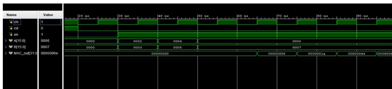
Fig 3. Timing diagram for coarse grained MAC
