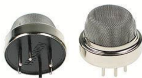
Fig -: Gas Sensor
