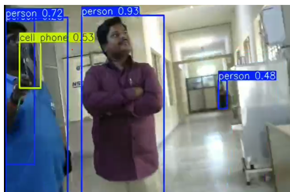
Fig. 3. Annotated detection output demonstrating YOLOv8 inference on embedded hardware with bounding boxes and labels
